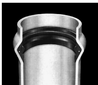
Rieber style gasket 2" through 8"
