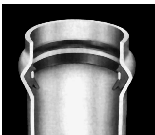
Retained Ring style gasket 10" through 24"
