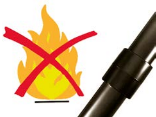
No open flames when cementing. No smoking.
