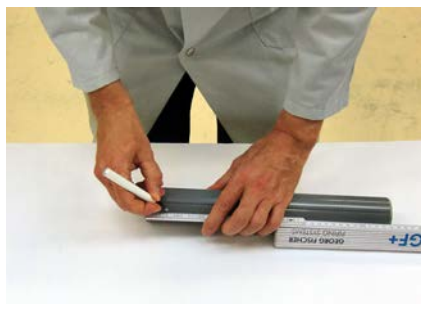
Marking the jointing length
