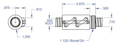
Ball bearing nominal diameter 1/8". Average ball quantity per nut is 168.
