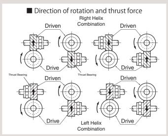
[NOTE] For parallel shaft applications, see the Application Hints for KHK Helical Gears (Page 167).
