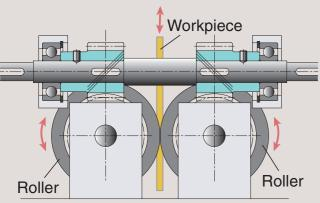
Rotate the rollers in reverse with one input shaft and move the pinched workpiece vertically
