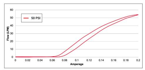
Calibrated with stabilized upstream pressure of 50 PSI to a flow of 50 SLPM @ 200mA.
