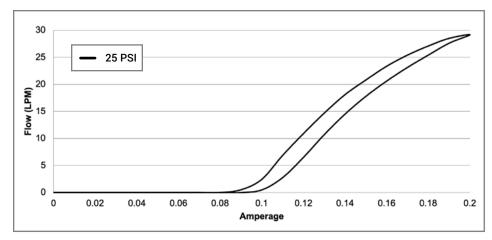
PV10PM2408050 will have precision control but less flow when upstream pressure is lower than 50 PSI. Typical curve with a stabilized upstream pressure of 25 PSI is shown.
