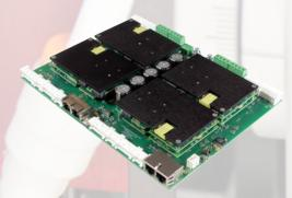
Optimum System Example: A single EtherCAT® slave node solution with 4 Axes of Motion and up to 280 Inputs and Outputs
