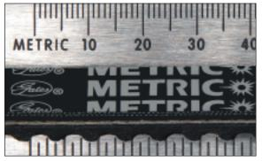
Classical V-belt sizes in the metric (DIN based) system are designated by a number followed by an "X" (10X, 13X, and 17X) followed by the length in millimeters (for example, 10X530).
