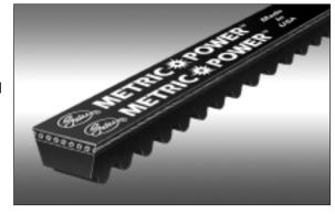
the Gates V80° matching system. This means each belt size is manufactured within a finite length tolerance so that any V80 belt will match and perform with any other V80 belt of the same length and cross section.
