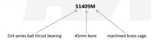
In this example a ball thrust bearing, series 514, with a 45mm bore, and a machined brass cage is described.
