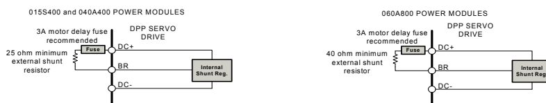
FIGURE 4.19 015S400, 040A400 and 060A800 Power Module External Shunt Resistor Connections
