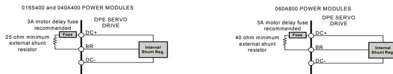
FIGURE 4.20 015S400, 040A400 and 060A800 Power Module External Shunt Resistor Connections
