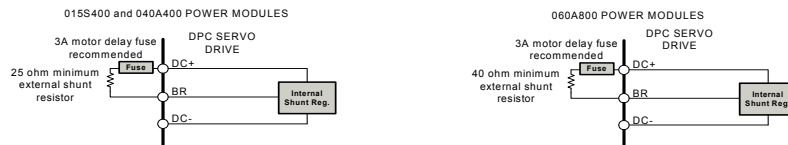
FIGURE 4.28 015S400, 040A400 and 060A800 Power Module External Shunt Resistor Connections
