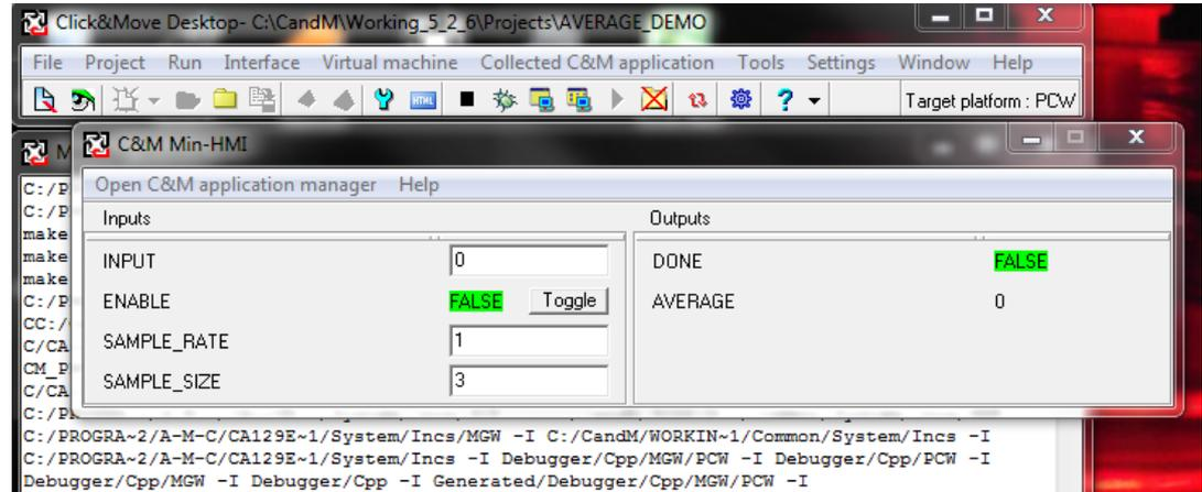
At startup the Min-Hmi will open with controls and indicators for each input and output on the main schematic.
