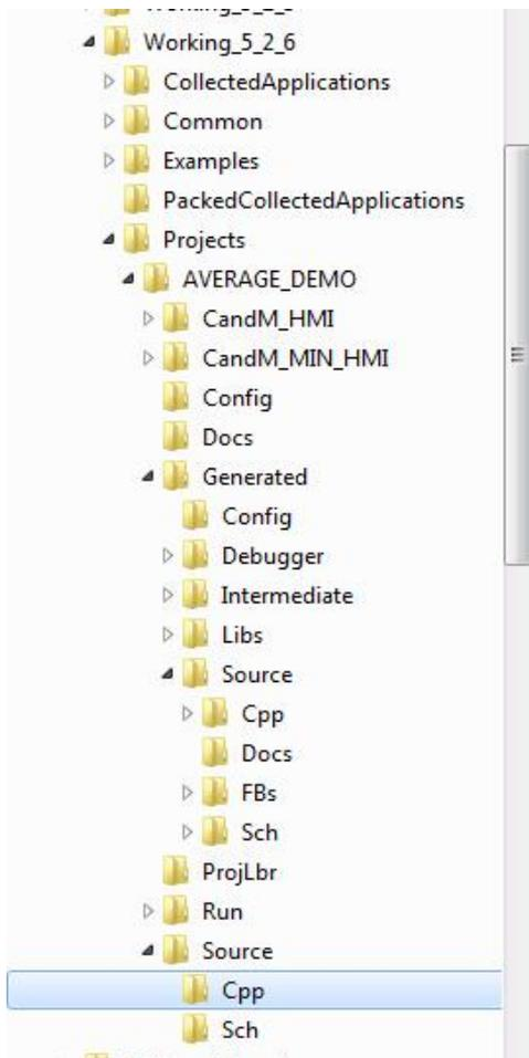
Create a folder named Cpp under the project\source folder. The new folder is shown in the image on the left. We must move the two files named CppAverageImpl.cpp and CppAverageImpl.h (Shown Below) from the project\Generated\Source\Cpp folder to the folder we just created. Be sure to move them, they must no longer exist in the Cpp folder under the Generated folder.
