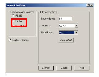
Once RS485 connection is established, the RS485 baudrate and drive address can be changed by pressing the connect icon on the tool bar and entering new values into the *connect to drive* dialog then pressing Connect.
