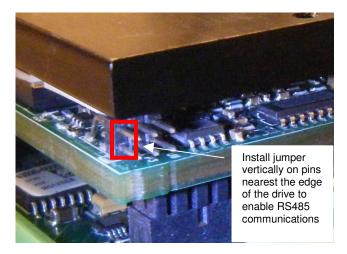
Once the jumper is installed, the drive must be power cycled to enable RS485 communications. The default RS485 communication parameters are *9600 baud* and *address 63* respectively.
