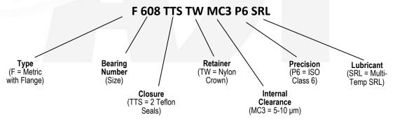
Note: No symbol for material code = high carbon chromium steel SAE 52100
